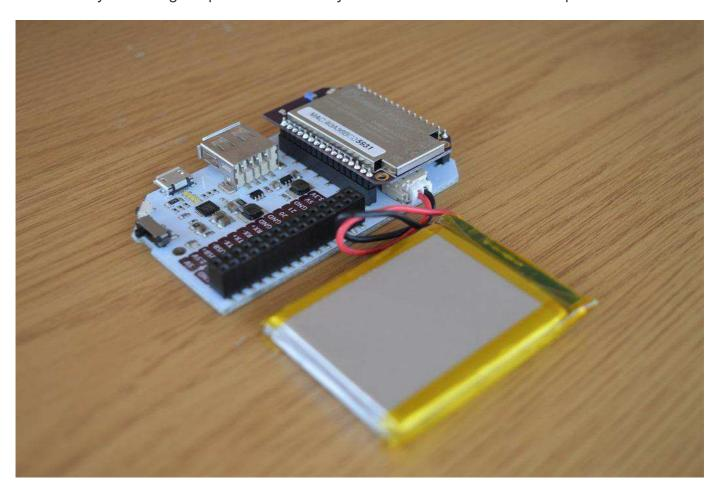
You may need to line up the pins with the holes before pressing the Omega into the Dock.
