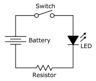
In the above diagram, the function of the Switch can be performed by a single relay.
