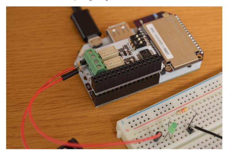
When we turn the relay on, it acts as a closed switch, allowing current to flow through the LED:
