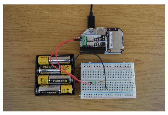
The positive lead of the battery pack is connected to the port labelled IN on the Expansion. A jumper wire is connected from the OUT port back to the circuit. Since the Relay is OFF, the switch is off and no current is passing through the LED:
