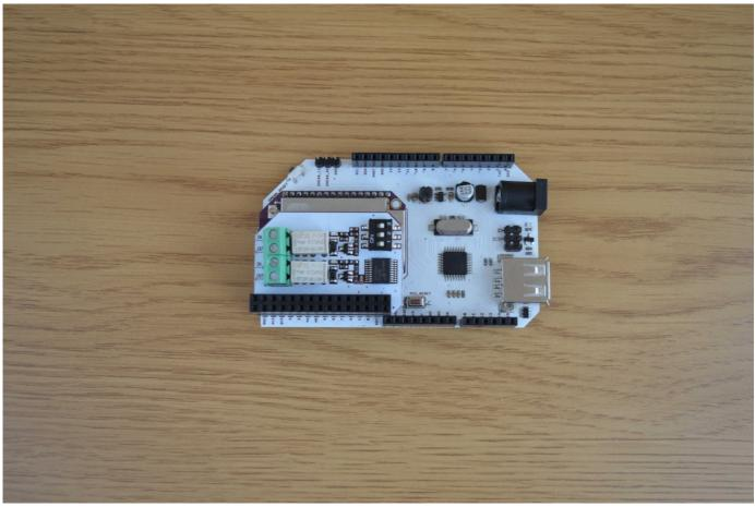
To connect the Relay Expansion to the Omega, plug it into the Expansion Header on the Expansion Dock.
