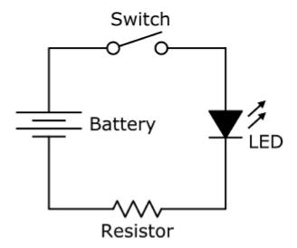
We can build this circuit without the switch:
