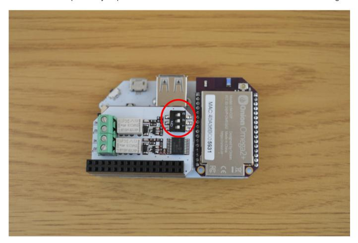
It has 3 switches that can be turned either ON or OFF. See the following table for the address values:
