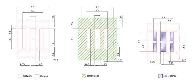
For superior solder joint connectivity results we recommend soldering under standard nitrogen atmosphere. Further information can be found in our Application Note: "Handling and Processing Details for Ceramic LEDs". Package not suitable for any kind of wet cleaning or ultrasonic cleaning.
