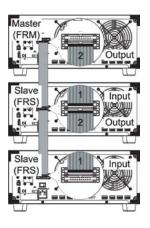
The PEL-2000A Series allows multiple mainframes to be linked together with standard MIL 20-pin connectors to provide higher power load capacity. A maximum of 5 mainframes, including one master and 4 slaves, can be chained together to give a 7kW load capacity for high current and high power applications
