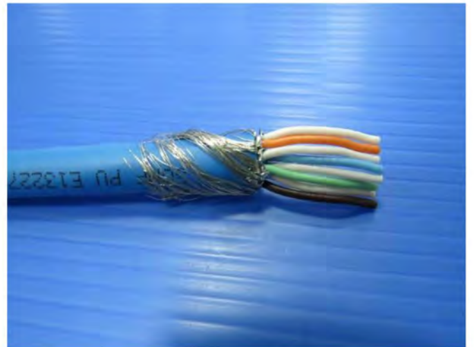
4. Cut off the foil and twist drain wire
