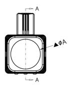
$\varnothing$ A= $\varnothing$ 8. 50  $\pm$  0. 10mm
