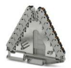
Potential distributors, Nom. voltage: 250 V, Nominal current: 17.5 A, Cross section: 0.14 mm² - 2.5 mm², AWG: 14 - 26, Connection method: Push-in connection, Number of positions: 2, Number of connections: 32, Width: 8.3 mm, Length: 100 mm, Color: gray, Color of connection elements: black, Assembly: NS 35/7,5, NS 35/15
