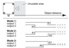
A1  $\rightarrow \infty$ , A2  $\rightarrow \infty$ : Object presence detection. Both outputs operate according to the selected mode, if an object is located within the detection range.
