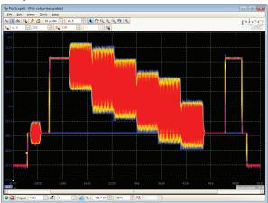
Advanced display modes allow you to see old and new data superimposed, with new data in a brighter color or shade. This makes it easy to see glitches and dropouts and to estimate their relative frequency. Choose between analog persistence, digital color, or custom display modes.
