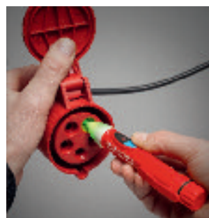
Phase sequence testing green = clockwise
