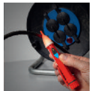
Testing of cable breaks
