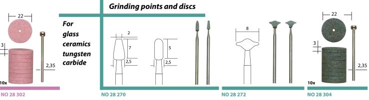
Silicon carbide grinding bits Fine particles of consistent hardness for engraving and frosting of glass, ceramics and stellites. Also for grinding tungsten carbide, chilled cast iron and other hard steel alloys. Shafts Ø 2.35.
