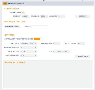
The VCP mode offers fully read and write access to all supported transponder types. The device can be operated via demo software, sample source codes, and a USB driver on Windows OS. Other operating systems are supported via a serial command protocol and a virtual ComPort interface based on a CH340E chip.
