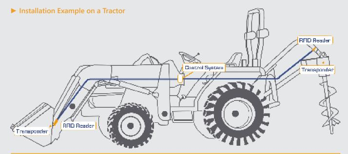
The cylindrical reader M30 is perfectly for the identification of attachements in agricultural machines. The antenna is mounted on the gripping arm of the vehicle. It identifies various external parts with attached transponder such as excavator bucket or drills. Next to the steering wheel is mounted a control system controller. The transponder contains data on the attached part and transports it with the antenna on the gripper arm to the control system.
