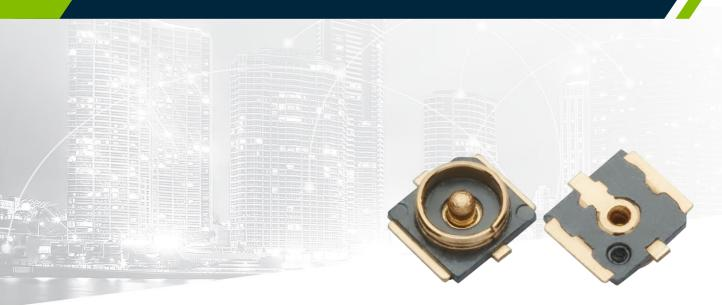
Part of the Taoglas TXR™ Series of receptacles, the TXR™ 4 RECE.20449.001E.01 is a 3-pad type wire-to-board SMT Receptacle solution that is ultra-small, lightweight and low profile, 1.6mm max. with an operational frequency range of DC to 6 GHz the TXR™ 4 RECE.20449.001E.01 is gold plated to provide superior performance and allow easy mounting of the male RF connector.
