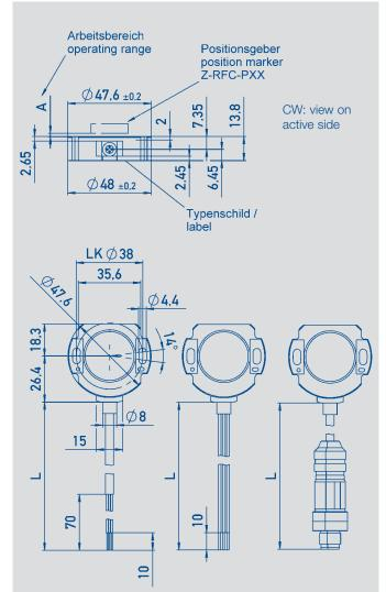
When the shaft marking is pointing to cable, the sensor is located in an electrical center position.
