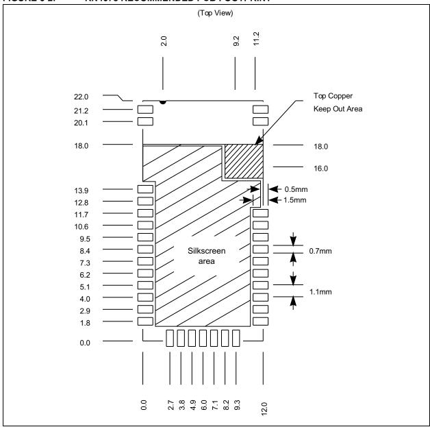
Figure 5-3 illustrates the recommendations for mounting the RN4678 on the host PCB, and also shows the minimum ground plane area to the left and right of the module for the best antenna performance.
