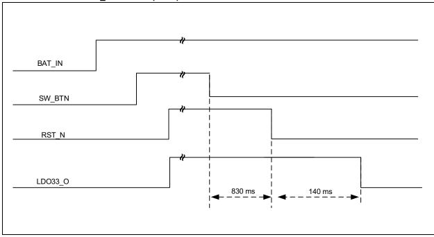
**Note 1:** 830 ms time duration is a typical value measured on iPhone<sup>®</sup> 6 and this time duration can vary from one smartphone to another.
