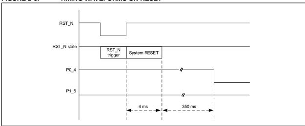
Note 1: The RST\_N state trigger must be greater than 63 ns.
