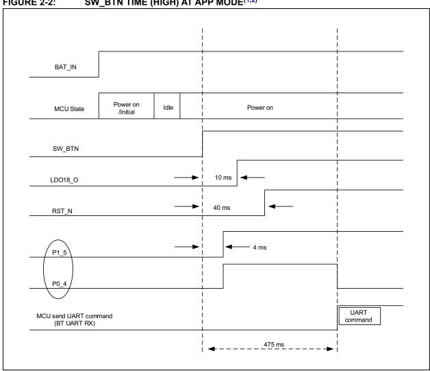
Note 1: Time duration (475 ms) is for reference purposes only. Use the Status Indication pins to verify the exact time when the host MCU can start sending the commands.
