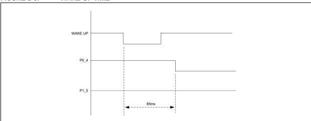
Note 1: The 85 ms is for reference time. Use the Status Indication pins to verify the exact results.
