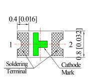
**Recommended Soldering Pad Dimensions**
