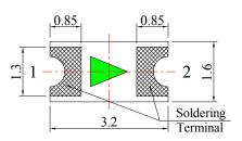
**Recommended Soldering Pad Dimensions**
