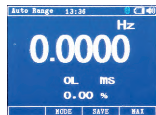
Frequency Measurement with Pulse Width and Duty Cycle
