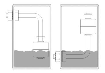
When mounted stem up, operating functions are reversed
