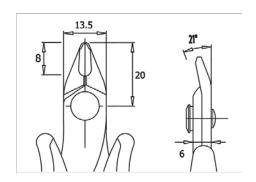
Suitable for cutting ferrous material
