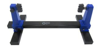
Robust PCB holder Sliding holder with screw fastening Surface area of base: 30 x 16.5 cm Working height: 11.5 cm Max. PCB width: 23 cm
