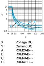
Note : These are typical curves, actual durability depends on load, environment, duty cycle, etc.
