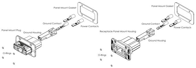
**ORDERING INFORMATION -** Color denotes signal or ground housings only. All other housings are black. Signal housings are available in 4 or 6 position styles. 6 position utilizes PPMX contacts. Ground utilizes ground contacts.
