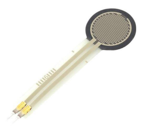
This is a force sensitive resistor with a round, 0.5" diameter, sensing area. This FSR will vary its resistance depending on how much pressure is being applied to the sensing area. The harder the force, the lower the resistance. When no pressure is being applied to the FSR its resistance will be larger than  $1M\Omega$ . This FSR can sense applied force anywhere in the range of 100g-10kg.
