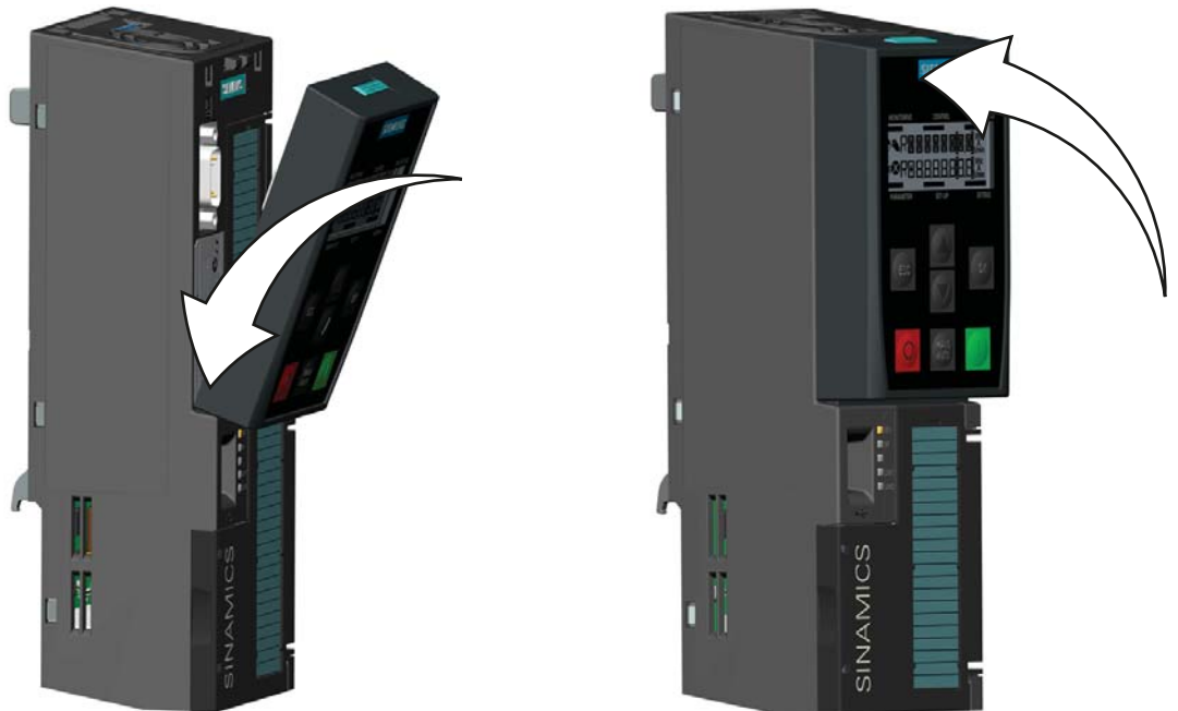
Figure 3-1 Fitting the BOP-2 to the Control Unit
