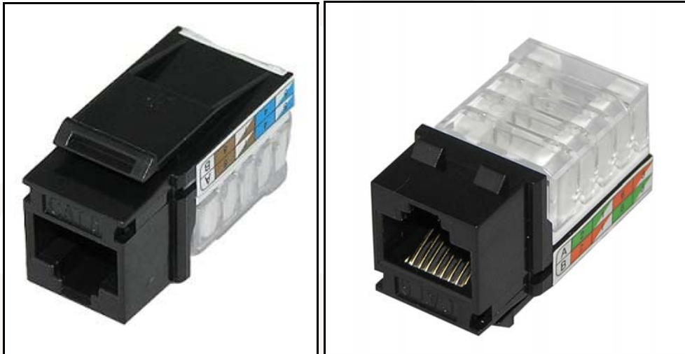
8p8c LSA+/110 dual IDC Category 6 component level keystone (SKmcbk/wh)
