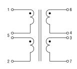
(Pin 1-2: 6-7 / short 3-4).....1:1 Insertion Loss (1-100 MHz) .....-1.5 dB max. Capacitance (Pin 5-3 / short 3-4) ......35 pF typ. Hi-Pot (Pin 1 to 6, short 3-4) Operating Temperature.....-40 to +85 °C Storage Temperature .....-40 to +85 °C Packaging ...... 2000 pcs. / reel
