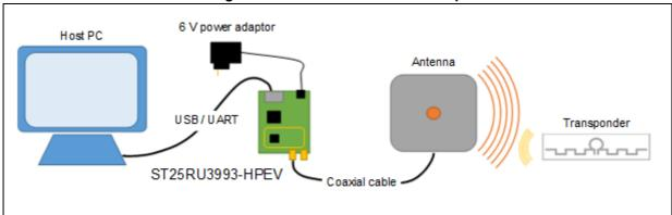
The host PC running the GUI is connected via a Micro-USB cable. The external power amplifier on the ST25RU3993-HPEV board is powered through the 6 V power adapter and must be connected when the external PA TX option is used. The antenna is connected to the active antenna port through a coaxial cable. A transponder is within the antenna range.
