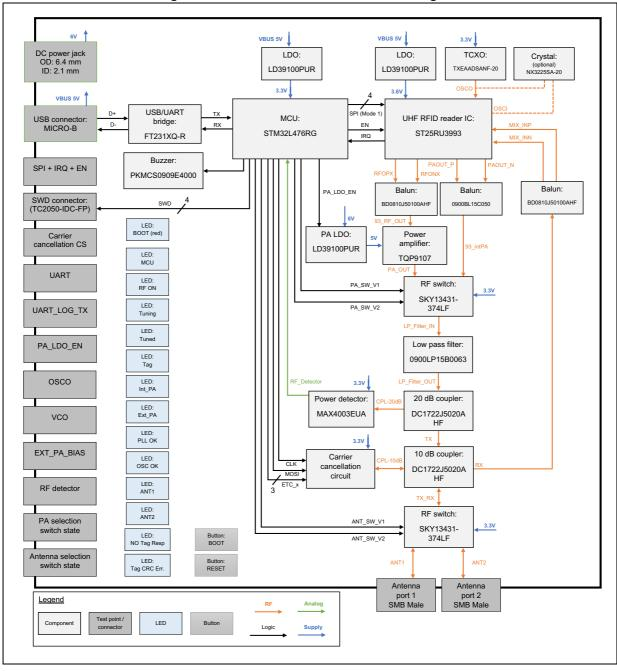
Figure 2. ST25RU3993-HPEV functional diagram
