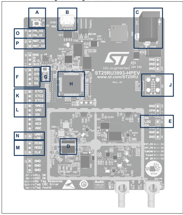
Figure 3. Main digital interfaces and buttons
