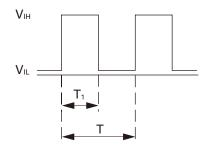
$V_{\text{IH}} = 4.75 \text{ to } 5.25 \text{ V} \quad V_{\text{IL}} = 0 \text{ to } 0.4 \text{ V}$   $PWM \text{ duty cycle (\%)} = \frac{T_1}{T} \times 100 \qquad PWM \text{ frequency } 25 \text{ (kHz)} = \frac{1}{T}$  Current source (Isource) = 1.0 mA max. (when control voltage is 0 V) Current sink (Isink) = 10 mA max. (when control voltage is 5.25 V)
