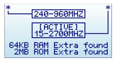
**Important**: Only one of the two SMA connectors is enabled at any given time. You select the active one using the Module option in the Frequency Menu, see page 15.
