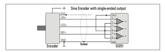
When the reference signals REF+ and REF- are not used or not available, the related inputs of the converter must be tied to a defined potential.
