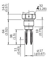
Housing (standard temperature range  $-40~^{\circ}$ C ... +100  $^{\circ}$ C), M12 x 1, IP67
