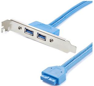
The USB3SPLATE 2-Port USB 3.0 A Slot Plate converts the USB pins on the USB 3.0 motherboard header to 2 standard USB 3.0 A-type ports. The plate can be mounted on the rear panel of a computer case, adding two USB 3.0 A female ports for simple connection to USB peripheral devices.
