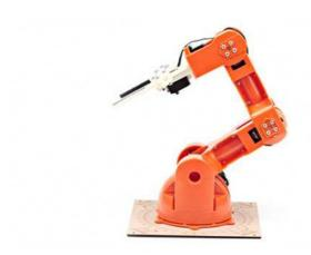
You can assemble your BRACCIO in a multitude of ways. Because it is designed for versatility, the BRACCIO can also support various objects on the end of the arm. The included BRACCIO shield allows you to hook up the servos directly to your Arduino board.
