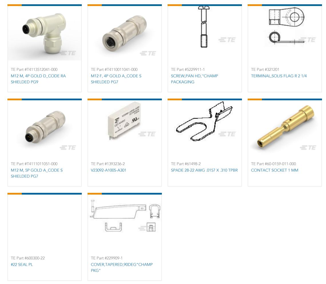
Standard Circular Connectors, Wire-to-Wire, 4 Position, Sealable, Wire & Cable, Signal, Nickel, Brass, D Polarization Code, M12 Connector
