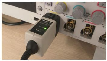
TekVPI probes communicate scale settings, ranges, and status to the TBS2000B.
