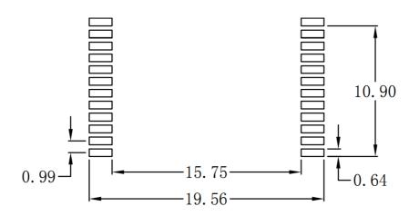
$\label{eq:Suggested Pad Layout}$  Dimensions are in millimeters with the following tolerances: X.XX =  $\pm 0.10$
