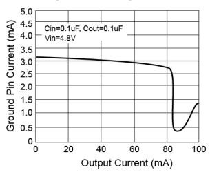
Figure 4. Ground Pin Current vs. Output Current
