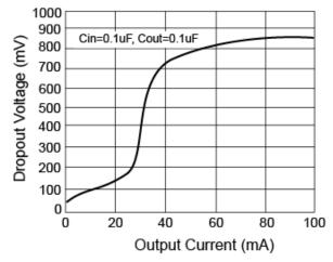
Figure 6. Dropout Voltage vs. Load Current
