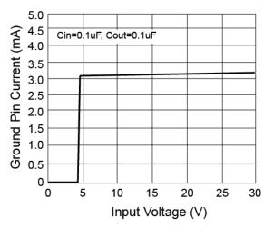
Figure 5. Ground Pin Current vs. Input Voltage
