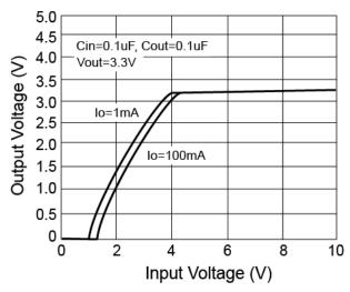
Figure 1. Output Voltage vs. Input Voltage
