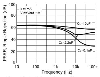
Figure 5. Ripple Rejection vs. Frequency
