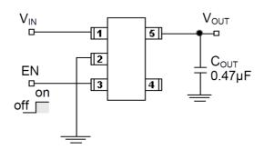
EN may be connected to  $V_{IN}$  pin to regulation ON  $C_{IN} > 0.1 \mu F$  in basic operating  $C_{OUT} > 0.47 \mu F$  in low noise operating
