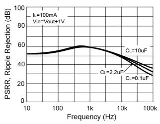
Figure 6. Ripple Rejection vs. Frequency
