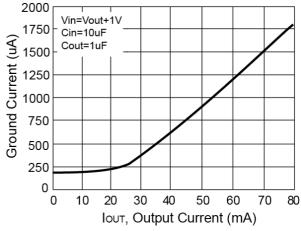
Figure 2. Ground Current vs. Output Current
