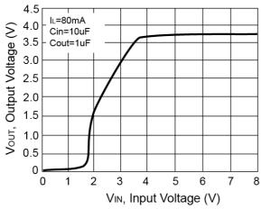
Figure 1. Output Voltage vs. Input Voltage
