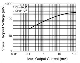
Figure 3. Dropout Voltage vs. Output Current
