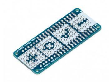
The **MKR Proto Shield** is a prototyping shield designed for your MKR board. This shield easily plugs onto your MKR using its provided female/male headers, and offers a duplicate breakout for each pin on the board along with many solderable through-holes on a standard 0.1" grid (2.54mm).
