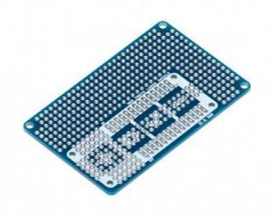
The **MKR Proto Large Shield** fits onto your MKR board using its provided female/male headers and enables you to fix it wherever you want with the mounting holes. This shield features a larger prototyping area with more than 300 solder points and makes connecting components to your board super simple, thanks to the silk that indicates the MKR board pins location
