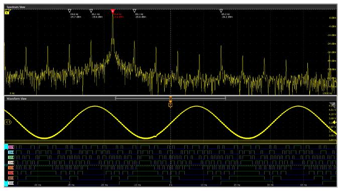
Beyond just analog and digital, FlexChannel inputs include Spectrum View. This Tektronix-patented technology enables you to simultaneously view both analog and spectral views of all your analog signals, with independent controls in each domain.
