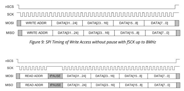
Figure 10: SPI Timing of Read Access with pause (tPAUSE) of 500 ns with fSCK up to 8MHz.
