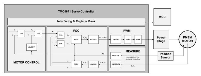
Figure 6: Hardware FOC Block Diagram
