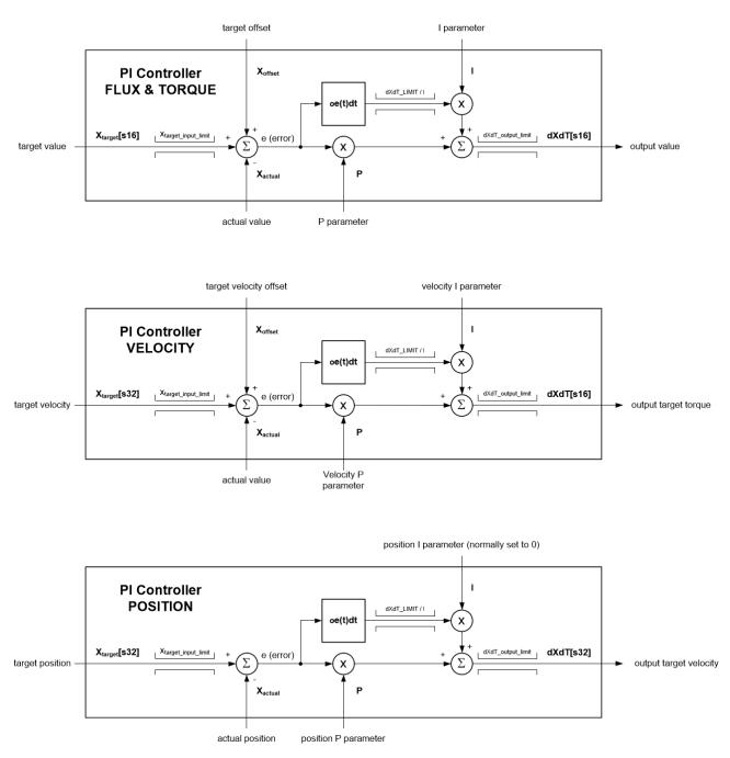
Figure 31: PI Controllers for position, velocity and current
