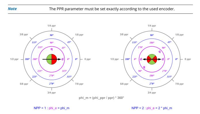
Figure 20: Number of Pole Pairs NPP vs. mechanical angle phi\_m and electrical angle phi\_e
