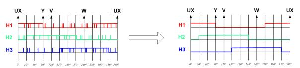
Figure 24: Outline of noisy Hall signals (left) due to electromagnetic interference with PWM switching and noise cleaned Hall signals (right) by PWM center synced sampling of Hall signal vector (H1 H2 H3)
