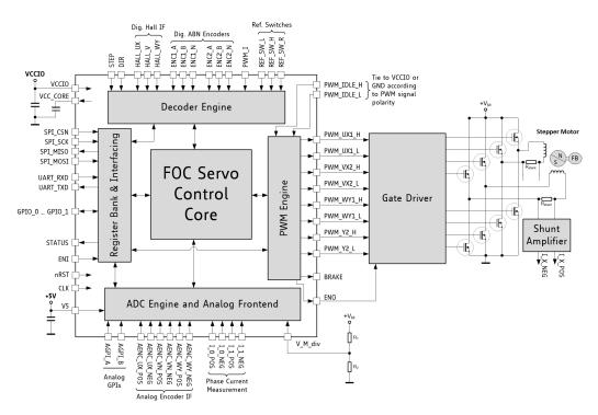
Figure 41: TMC4671 Pinout with Stepper Motor
