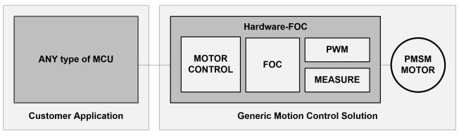
Figure 5: Hardware FOC Application Diagram
