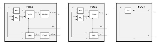
*Figure 38: FOC3 (three phase motor), FOC2 (two phase stepper motor), FOC1 (single phase DC motor)*
