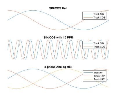
Figure 27: Analog Encoder (AENC) signal waveforms
