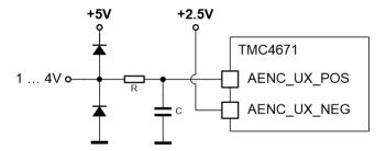
Figure 44: Sample Circuit for Interfacing of a single ended analog signal
