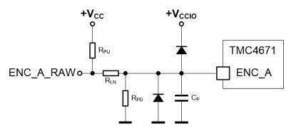
Figure 43: Sample Circuit for Interfacing of an Encoder Signal
