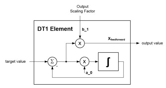
Figure 36: DT1 Element Structure
