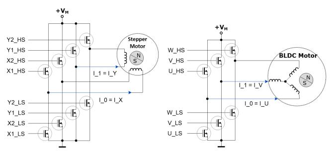
Figure 45: Phase current measurement: Current directions for 2 and 3 phase motors
