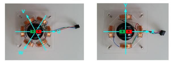
Figure 4: Compass Motor Model w/ 3 Phases UVW (FOC3) and Compass Motor Model w/ 2 Phases (FOC2)
