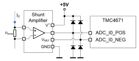
Figure 47: Current Shunt Amplifier Sample Circuit
