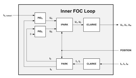
Figure 32: Inner FOC Control Loop
