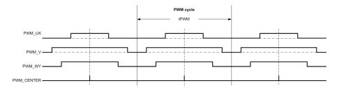
Figure 25: Hall Signal PWM Center Sampling on PWM\_CENTER
