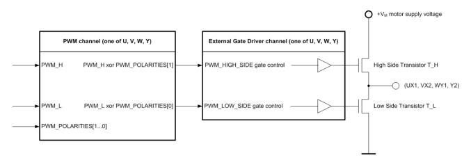
Figure 37: PWM Gate Driver Control Polarities
