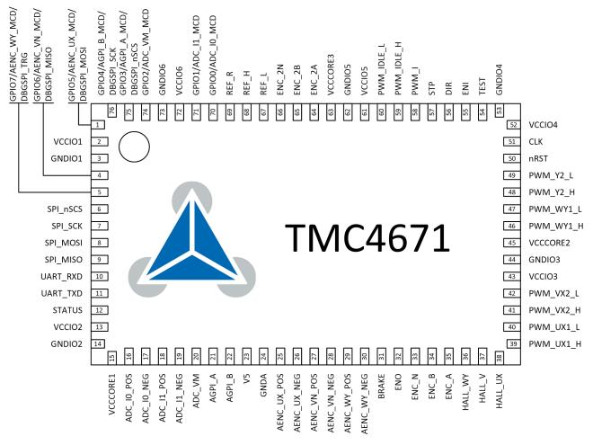
Figure 49: Pinout of TMC4671 (Top View)
