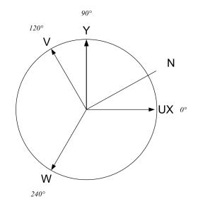
Figure 21: ABN Incremental Encoder N Pulse
