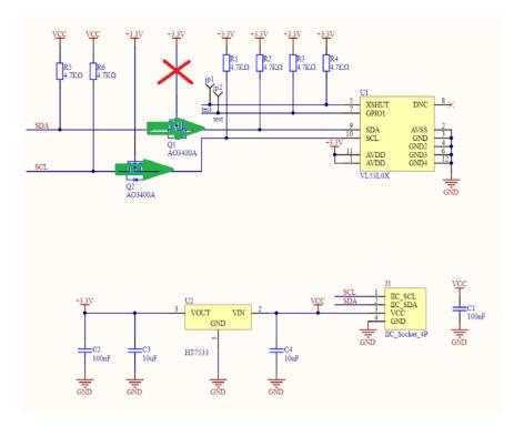
In this case, make sure you use the 3.3V on SDA and SCL, M5Core GROVE provide 3.3V to data pins, 5V to power pin. only 3.3v allowed on VL53L0x.
