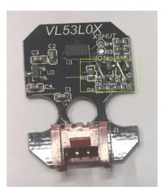
• If not, take off the two MOSFETs (AO3400A), and connect SCL,SDA from GROVE directly to SCL,SDA on
