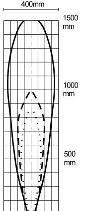
Beside the three typical cone shapes for the UPR-A sensors are shown (small, medium and large cone). Furthermore, the size of the detection beam is influenced by air temperature and humidity. The colder and dryer the air, the larger is the beam.
