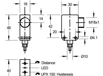
Use the miniature screw driver which is included for adjustment of the two potentiometers.
