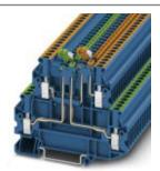
Knife disconnect terminal block, With test socket screws for insertion of test plugs, Connection type: Screw connection, Cross section: 0.14 mm² - 4 mm², AWG: 26 - 12, Nominal current: 16 A, Nominal voltage: 400 V, Length: 80.1 mm, Width: 5.2 mm, Color: blue, Assembly: NS 35/7,5, NS 35/15
