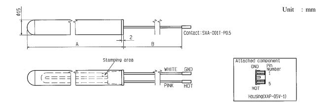
\* The housing that connect with the edges of wire harnesses, will be attached as a another part of this assembly. (Due to easy to assemble this product to your product that needs water proof design with O ring. : Please see page P.12.)
