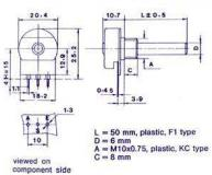
20mm rotary carbon track potentiometers for PCB mounting. Metal/plastic housing and plastic axe ( $\varnothing$  6mm). Optional single-pole switch (1A-24Vdc / 0.3A-250Vac).
